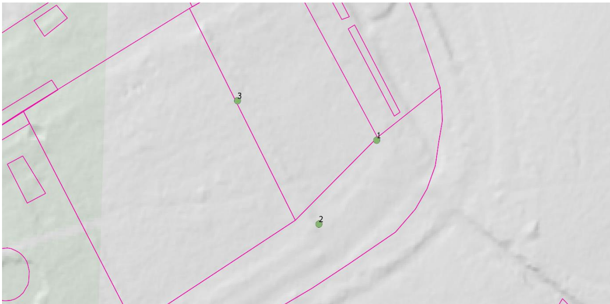
Figure 5. GPS point on the LIDAR confirming wall alignment
